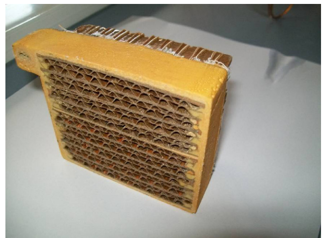
Fig. 3. End fragment of the moulded honeycomb block after the cutting of about 25 grids.
